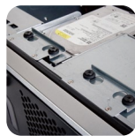
Anti-vibration drive cage design
